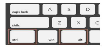
**Use:** A special key, in the context of computing and technology, refers to a keyboard key that performs a specific function beyond the standard alphanumeric input. Examples of these include keys like Control (Ctrl), Alt, Shift, Function (Fn), Escape (Esc), and the Windows key on a Windows-based computer.
