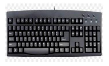
A **keyboard** is one of the primary input devices used with a computer. Like an electric typewriter, a keyboard is composed of buttons to create letters, numbers, and symbols, and perform additional functions. Keyboard is used for entre a text, numbers and Different symbols. Some keyboards are wired or some keyboards are wireless.
