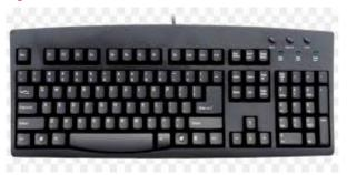
A computer keyboard is an input device that allows a person to enter letters, numbers, and other symbols (together, these are called characters) into a computer. It is one of the most used input devices for computers. Using a keyboard is often called typing.
